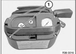
Release hexagon nut (1), grip nut firmly from underside.
